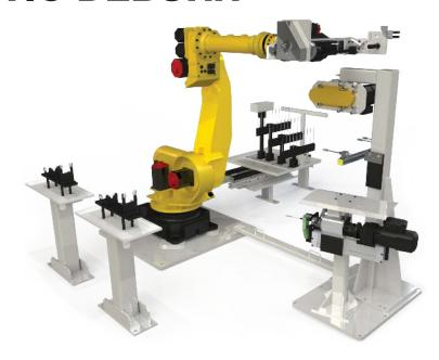
LOOKING FOR THE ULTIMATE IN DEBURR and debris removal agility? Look no further. FLT'S Robotic Deburr comes fitted with multiple brush configurations including a long bottle brush for hard to reach locations. It has a chamfer tool and a blow off station for metal chip removal. Tool change is automatic and it comes equipped with brush sensors for error proofing.
