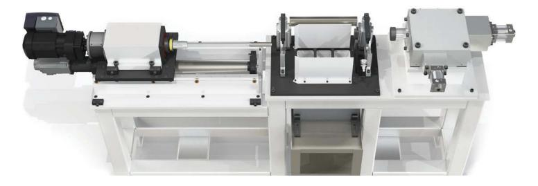
FLT'S DEEP REACH DEBURR SOLUTION IS BUILT TO HANDLE A WIDE RANGE of automated deburr tasks, including uneven and multifaceted surfaces. Irregular edges are cleaned and smoothed while advancing and retracting, reducing cycle time.
